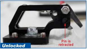
**STEP 3:** The latch assembly needs to be squared and centered with the striker plate. Move the striker plate side to side to center. Make sure striker plate remains parallel with opposite striker plate.
