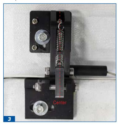
**STEP 4:** Move the latch assembly forward or backward to obtain proper engagement. To move the latch, you need to loosen the ¼-20 locknut on the roof bolt. The latch assembly needs to be far enough forward to ensure proper engagement. Once everything is in place, tighten the 1/4-20 locknut.
