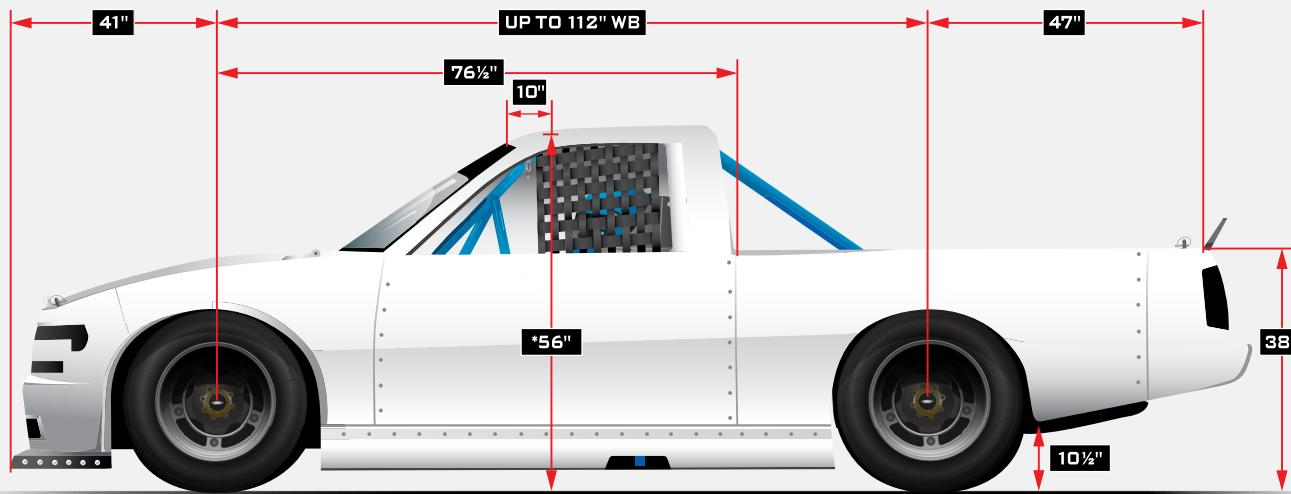
NOTE: 79 1/2" Width at Wheel Openings & \*The Roof Height is measured 10" back from leading edge of roof.
