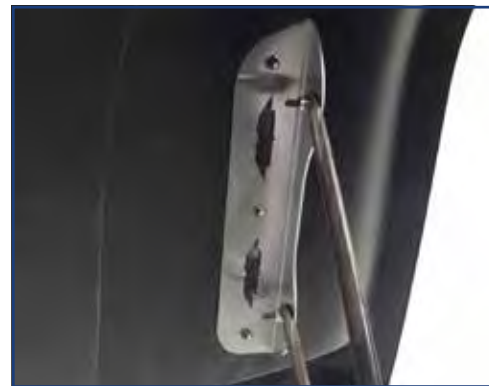
11002-75333: MOUNT VERTICALLY ON NOSE SIDE
