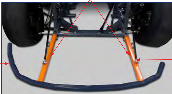
FRONT BUMPER MOUNTING KIT (HIGHLIGHTED IN ORANGE) WITH BLACK ADJUSTABLE BUMPER SUPPORTS
