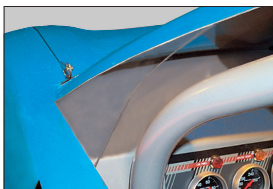
THE 000-6202 DOOR VENT WINDOW IS OVERSIZED; TRIM TO FIT YOUR APPLICATION
