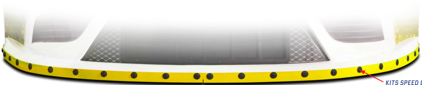
11002-41551-Y YELLOW WEAR STRIPS FULLY INSTALLED WITH 00001-72651 UNIVERSAL BODY MOUNTING KIT
